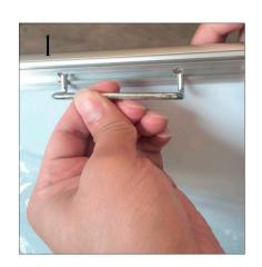
Snap open frame and insert slat wall attachment into snap frame as per image 1.
