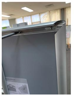
Stop at a desired height and tighten the screws from inside the frame. Please see image above.
